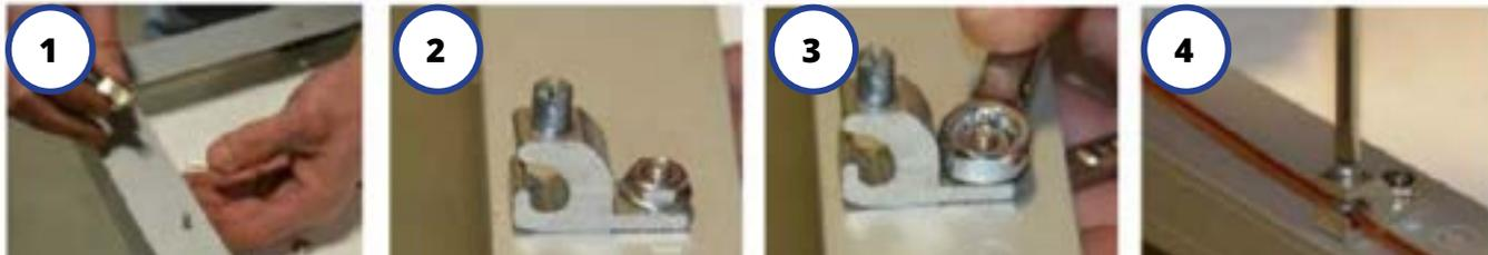
Install ground lug on the module per ground lug and module manufacturer's instructions
